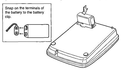
off "Lo" flashes for over 10 seconds after installing a new battery, disconnect the AC adaptor and reinsert it again without removing the battery. "Lo" flashing will disappear after 10 seconds.
